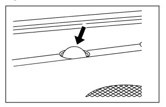
The light sensor for the DRL and AUTO headlamp feature is located on top of the instrument panel. If you cover the sensor, it will prevent it from sensing light, and the exterior lamps may come on whenever the ignition is on.
